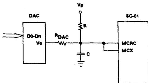
Figure 7. Variable Voice by DAC Current Injection
