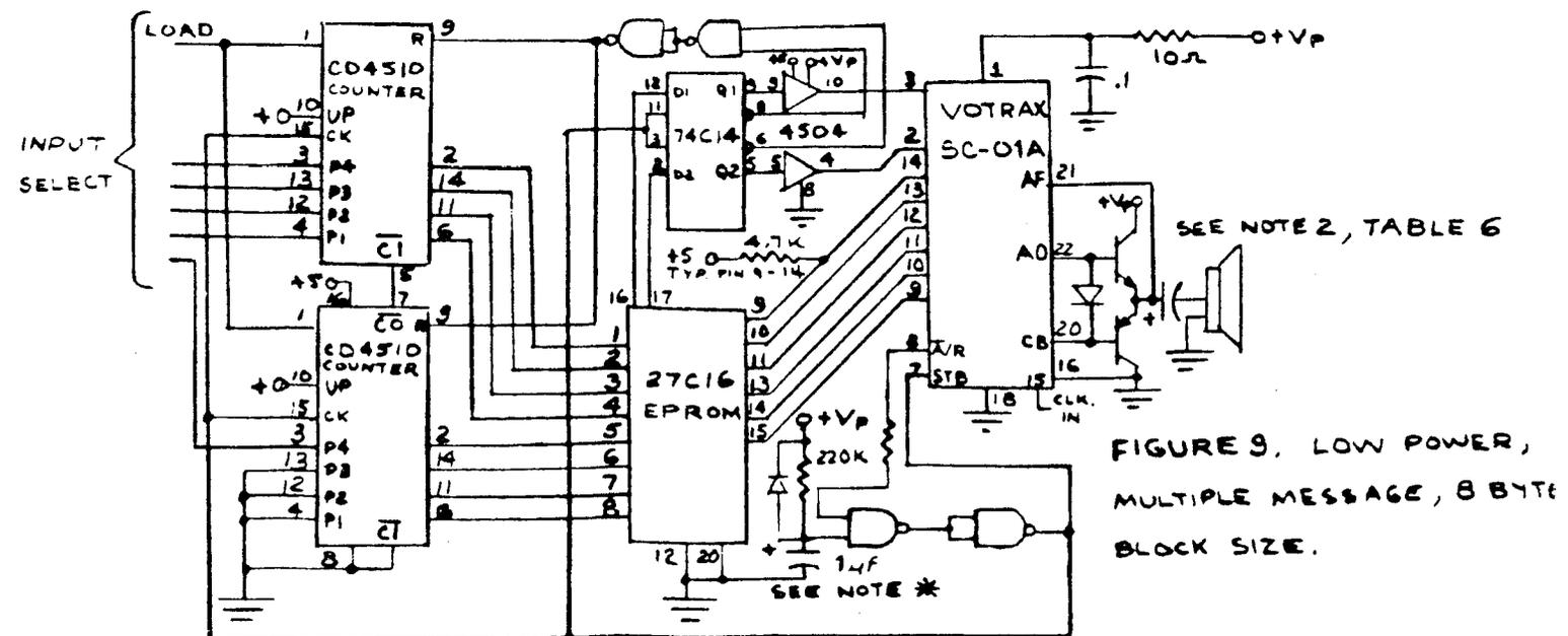
FIGURE 9. LOW POWER, MULTIPLE MESSAGE, 8 BYTE BLOCK SIZE.
