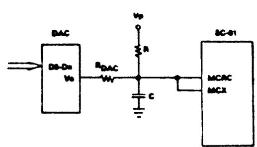
Figure 7. Variable Voice by DAC Current Injection
