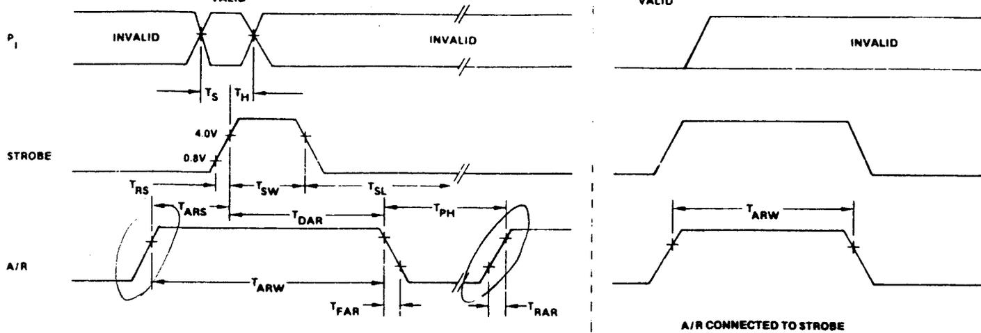
Figure 4. Timing Diagram
